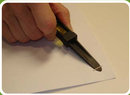
Slide remover end under staple to remove it
